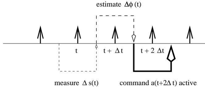
FIG. 4.1. Time line for a 2-cycle delay AO system
