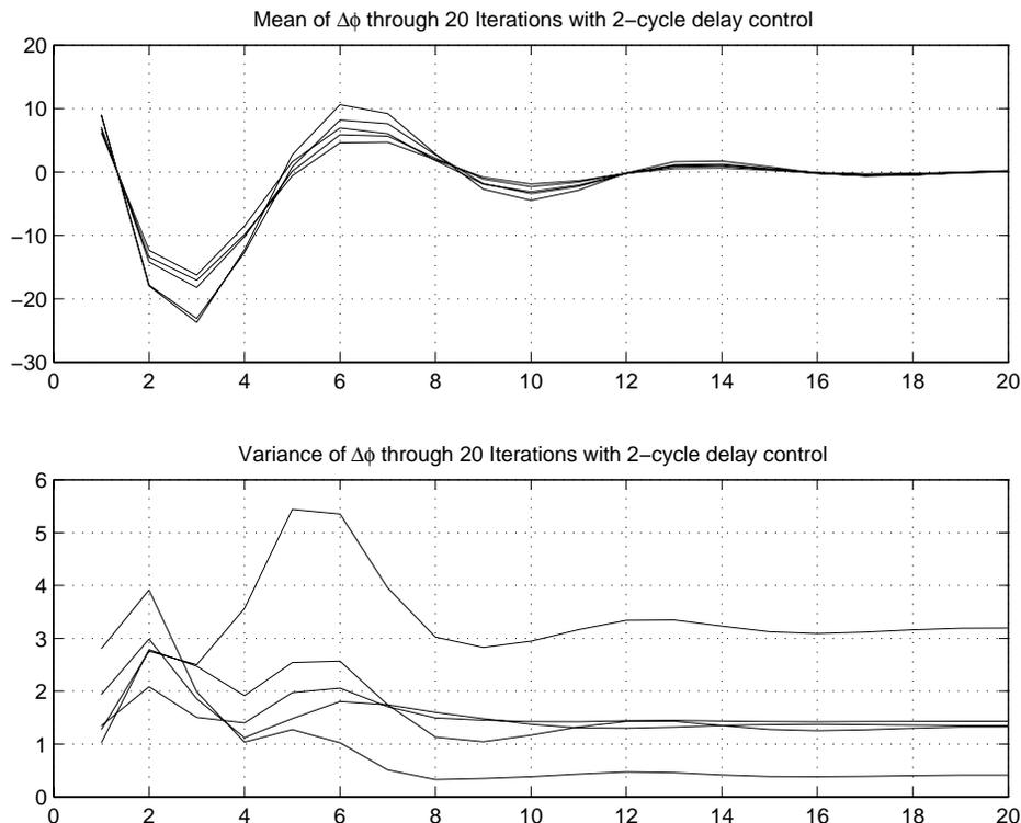
FIG. 5.3. Convergence of  $\Delta\phi$  with 2-cycle delay control (4.21)
