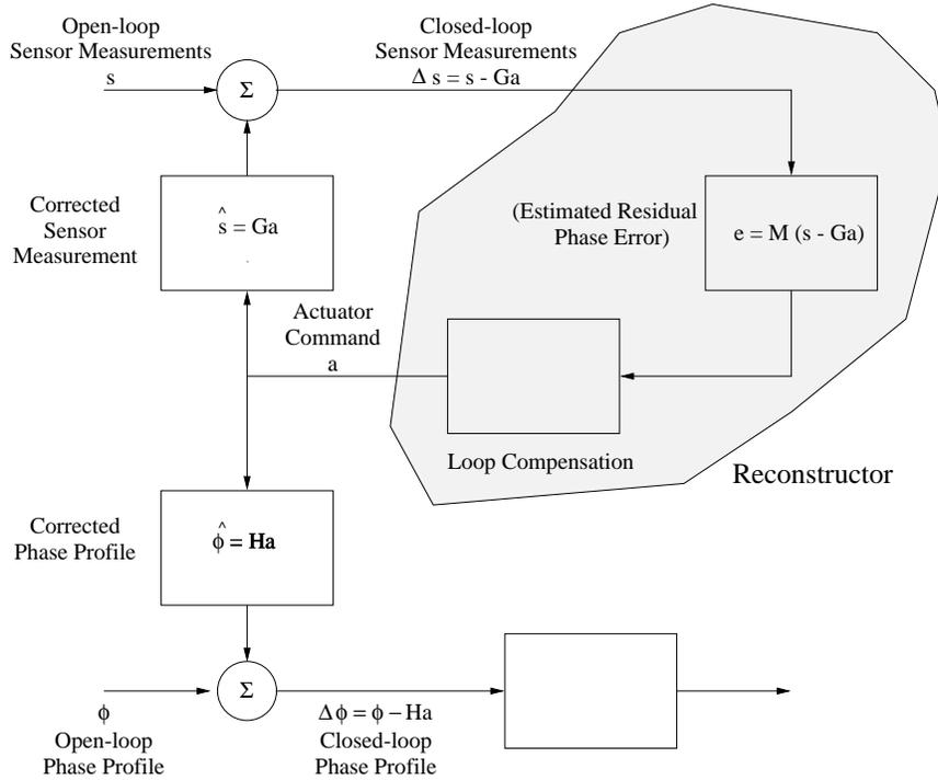
FIG. 3.1. A close-loop AO control model
