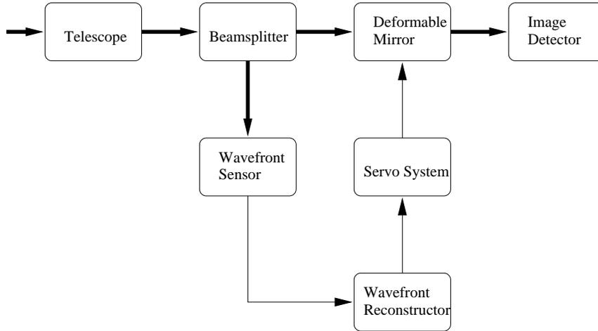
FIG. 3.2. *An open-loop AO configuration*
